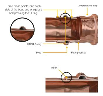
On fittings 1/2" and upwards, a hook ensures that the high pressure performance achieved by >B< MaxiPro fittings is maintained.
